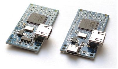
The one on the left is the legacy Pluto-IIx HDMI (TXDI serial interface). The one on the right is the new Pluto-IIx HDMI (USB-C serial interface).
